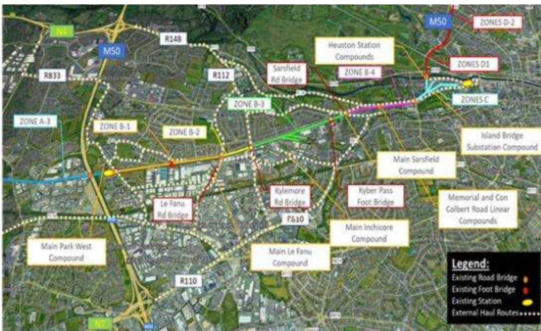
Figure 5-41 Construction Zone B: External Haul Routes
