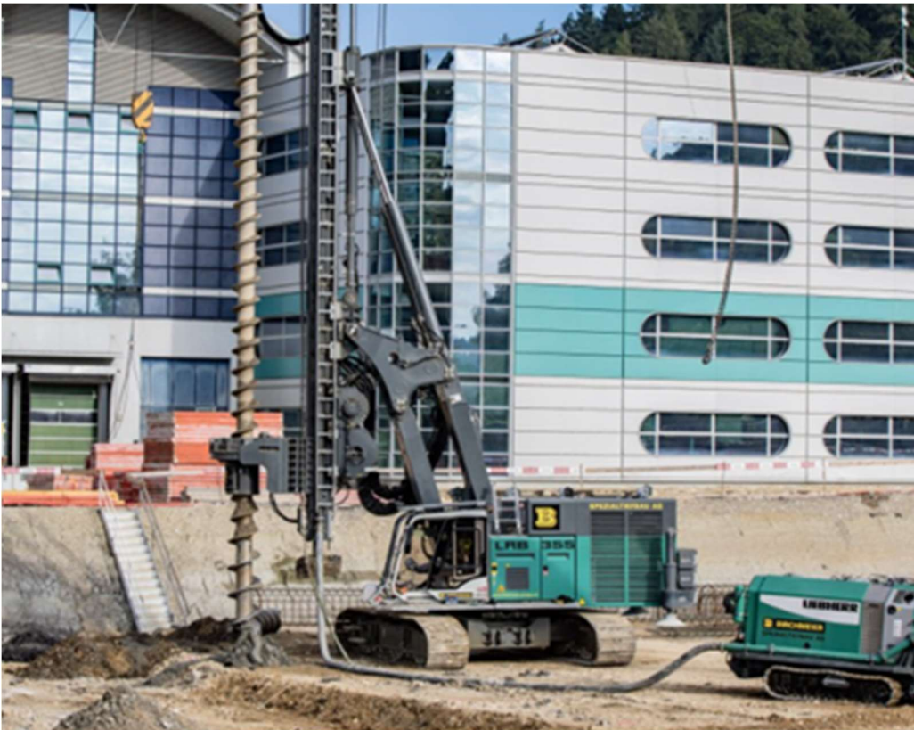
Figure 5-5 Example of CFA Piling Rig
