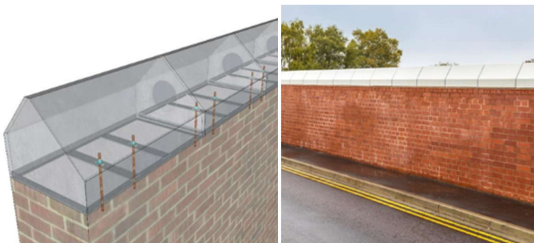
Figure 5-20 GRP Parapet Extension
