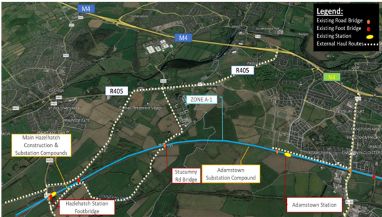
Figure 5-38 Construction Zone A-1: External Haul Routes
